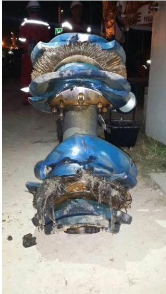
Cleaning Pig Damage
