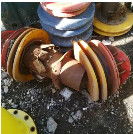
Damaged Cleaning Pigs
