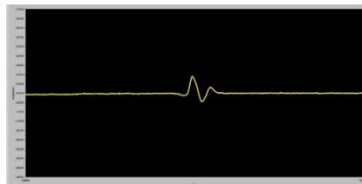
Crack buried at 6mm
