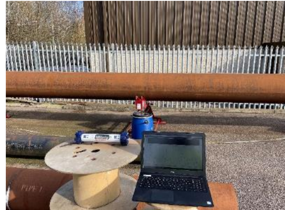
EMRx positioned 1m from pipe centre
