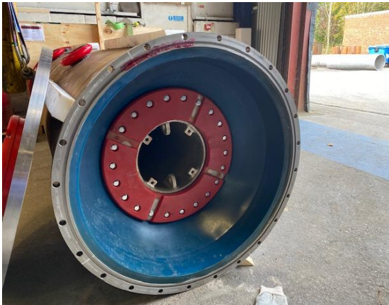
Figure 15: Operational Pigs Loaded into Cassette
