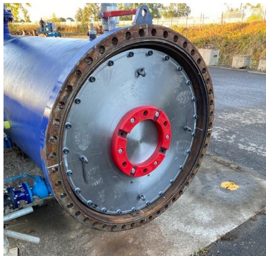
Figure 17: Cassette loaded into Test Rig
