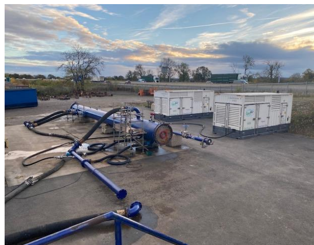
Figure 12: Air Testing Set Up
